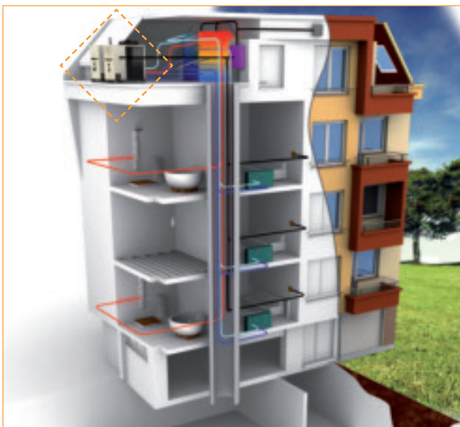
Example of GAHP-AR applications in winter and summer operation with radiant panels, fan coils and indirect production of DHW.
