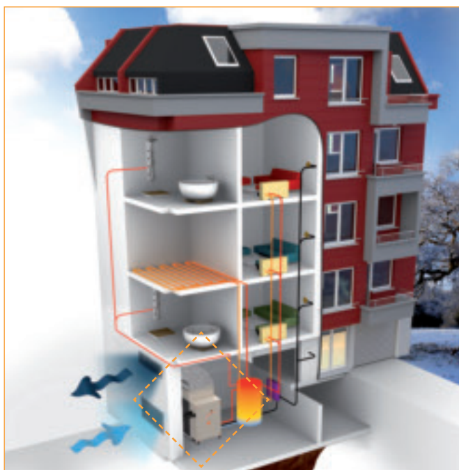
Examples of GAHP-A Indoor application in the plant room.
